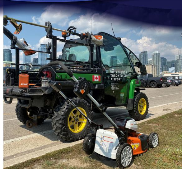
Billy Bishop Airport has replaced gas-powered equipment for grass and vegetation control with battery-operated technology in an effort to reduce the emissions from its fleet of maintenance equipment.
