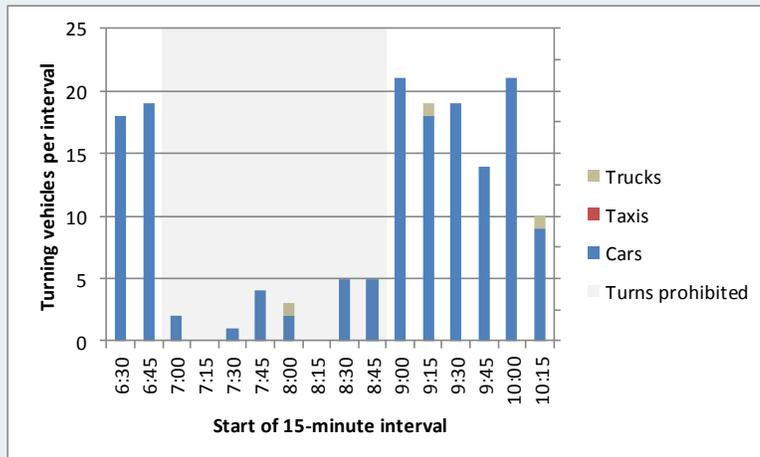
During the morning, a minor number of vehicles were observed violating the eastbound right turn prohibition — an average of ten per hour between 7:00 and 9:00, or approximately one vehicle every two to three cycles. No taxis were observed making this movement. This is roughly comparable to the spring 2015 observations.
